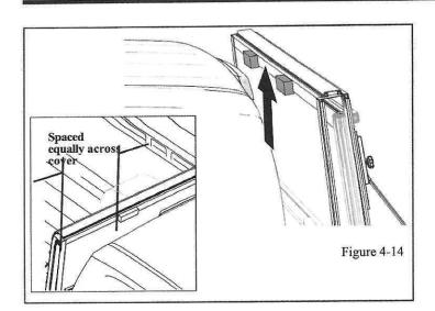
(n) Install the two cab bumpers along the top edge of the cover equally spaced from left to right. (Figure 4-14)
