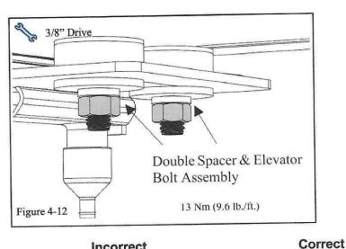
(1) Carefully fold the cover forward and tighten the four (4) hex nuts to 13Nm (9.6 lb./ft.) and ensure that the lock washers are completely flat. (Figure 4-12)
