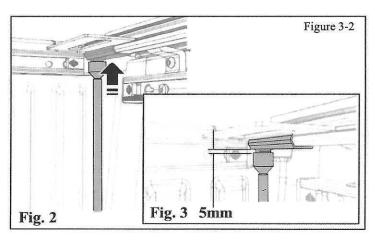
(b) Slide the drain hose adapter with the drain hose onto the drain cap until it stops. (Fig. 2) There should be approximately a 5mm gap between the top of the drain adapter and the bottom of the drain cap. (Fig. 3) (Figure 3-2)
