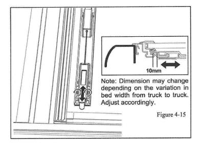
(o) The cover panel latches can also be adjusted by loosening the mounting screws and moving the latch assembly out or in to better engage the cover side rail. Re-tighten the screws. (Figure 4-15)
