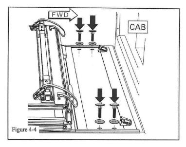
(d) Insert the elevator bolts through a rubber washer, through the front panel and through the slotted bracket, one each side (Figure 4-4).
