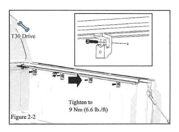
(b) Mount the bed cover rail into the holes in the truck bed from the cargo rail. Reuse the fasteners from step 2. Before tightening, make the necessary adjustments to the rail so that is pushed forward and tight against the front bulkhead. Then tighten screws to the recommended torque of 9Nm (6.6 lb./ft) (Figure 2-2)
