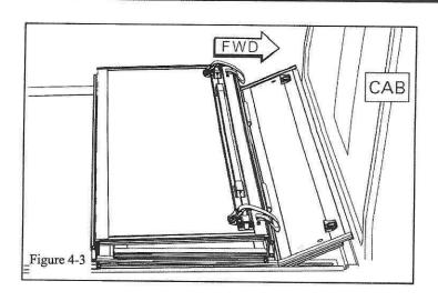
(c) The front panel folds down over the slotted rail brackets. The front panel must sit just inside the bulkhead rail with the seal resting on top of the bulkhead. Fold the panel down and align it so it sits squarely on the rails and align the mounting holes with the slotted rail brackets (Figure 4-3).
