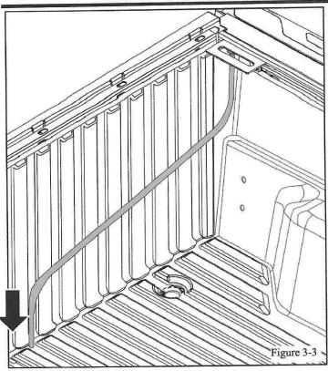
(c) Install the drain hose on the bottom of the truck bed, through the hole nearest the bulkhead and nearest the center of the bed. Mark the drain hose anywhere between 50 to 80mm from the hose end to ensure the drain hose extends below the hole in the truck bed. Install the drain hoses on both sides of the bed. (Fig 3-3)
