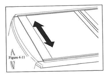
(k) Adjust the cover side to side to make sure latches make proper contact with the rails. (Figure 4-11)
