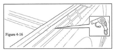
(p) The side seals may appear wrinkled shortly after installing the cover, they will flatten out over time. Or, a hair dryer, heat gun or exposure to the sun will help to smooth them. (Figure 4-16)
