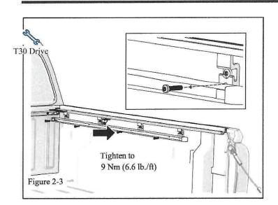
(c) Mount the cargo rail to the 'S' clamps through the lower hole in the clamp. Use the screws from the hardware bag. Tighten to 9Nm (6.6 lb./ft) (Figure 2-3).
