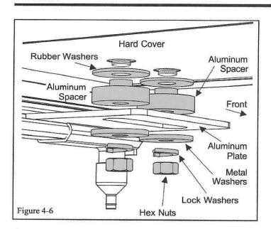
(f) Assemble the metal washer and lock washer onto the elevator bolt from underneath the slotted aluminum plate. Then **loosely** install the hex nut (Figure 4-6).
