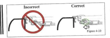
(j) Check to see that the cover panel latches make proper contact with the side rails (Figure 4-10).
